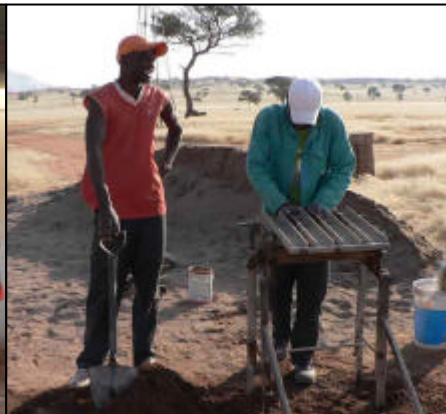
Using the Wolwedans brickmaker, bricks are made on site
